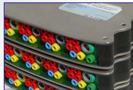
Multiple units of g-USBamp can be stacked to set up a multi-channel system. All channels are sampled synchronously.
